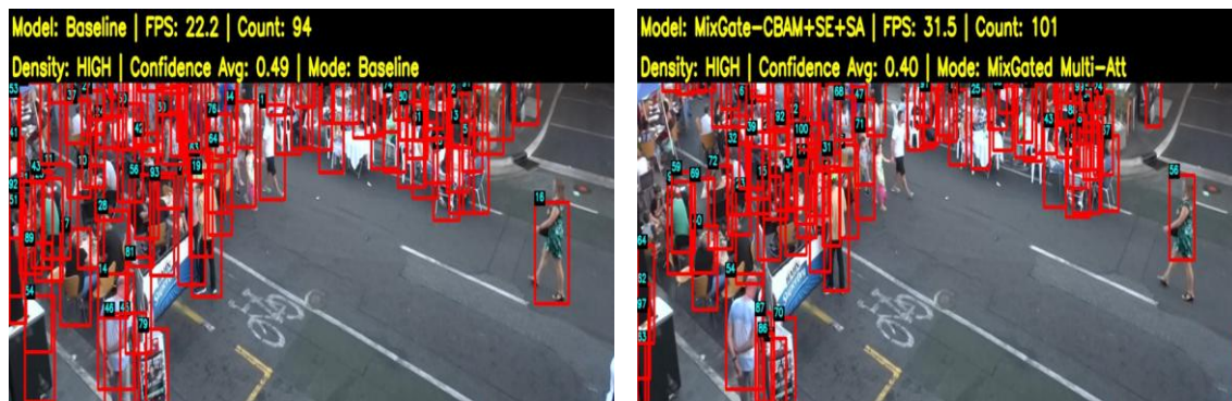
Figure 8 Qualitative comparison of detection results on the MOT20Det dataset: (a) Baseline YOLOv11s; (b) Proposed Mix-Gated-CBAM+SE+SA.
